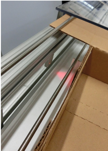
A through-beam sensor, shown here, is the most reliable method for indicating a part is present.
