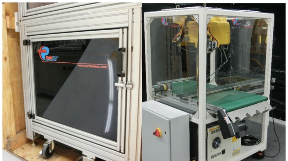
A comparison of a machine built using an aluminum frame (left) versus a machine using a steel base (right)
